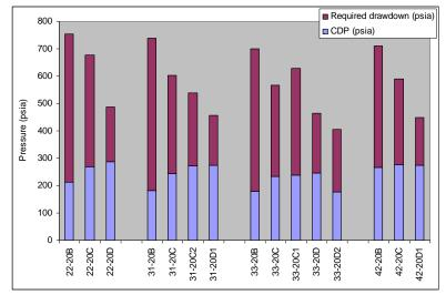
Figure 3 - Plot of critical desorption pressure and required drawdown by well pad
