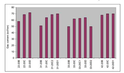
Cook and Anderson coal seams contained more gas and less water than the deeper Wall seam. In addition, the tests revealed that critical desorption pressure and gas content varied to a surprisingly high extent between coal seams and, within each coal seam, between well pads.
