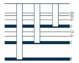
Figure 1 (Left) is a diagram of the three well pod structure used in this study. The study area was focused on four well pads that straddle the Powder River. Each well pad included three wells that were completed initially in three different coals the Anderson, the Cook and the Wall seams (Figure 1 above). Above each of the Anderson and the Cook seams were present up to three stringers of the base coal seams. The four well pads in Section 20 were configured in a diamond pattern.
